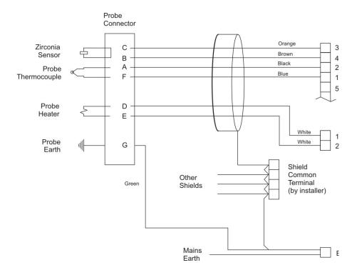
Figure 3-4: Model 9060L Heated Probe Cable Connection
